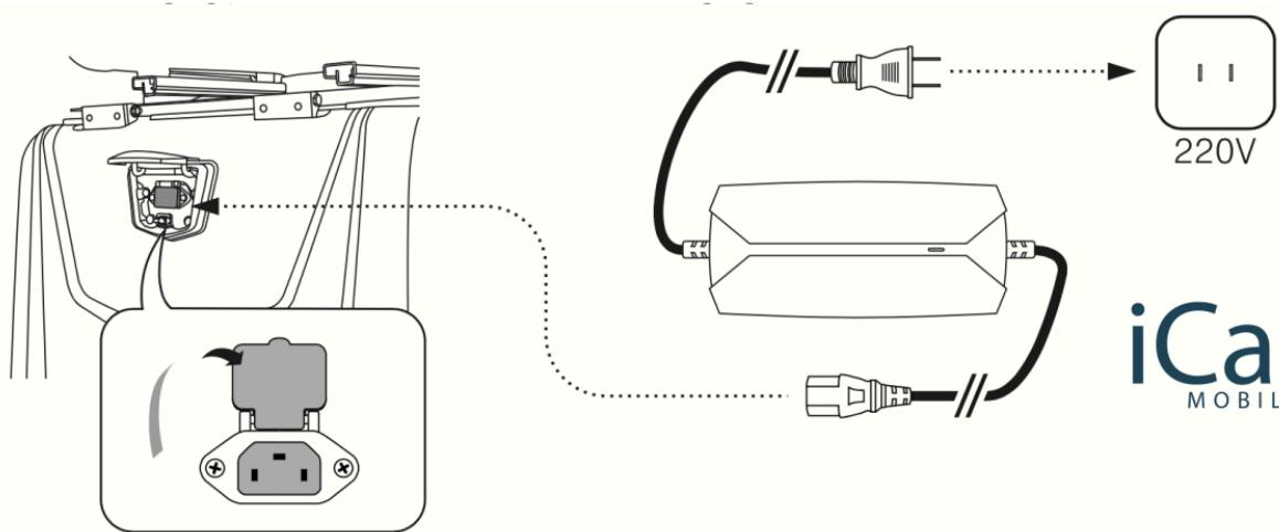
The charger is designed to operate safely within a voltage range of AC  $220V \pm 20\%$ . Operating outside this range may result in undercharging the battery or damaging the charger.
