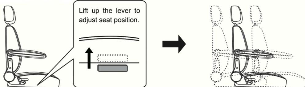
**Ensure that the seat and backrest are securely locked in position after making adjustments.
