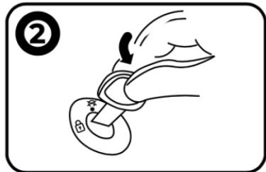
To turn off the steering wheel lock, **push** the key into the ignition and turn it clockwise to the 'OFF' position
